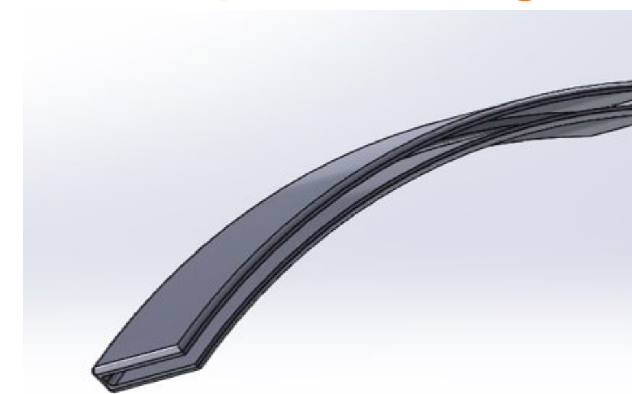
Fig3: The thin adaptor can easily clip on and off from the laryngoscope. It is single-use, and disposable.
