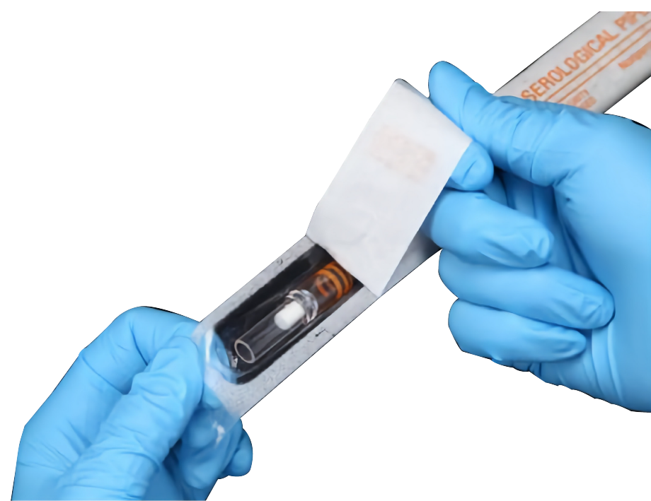
Figure 1. Manufacturer Suggested Pipette Opening Technique
