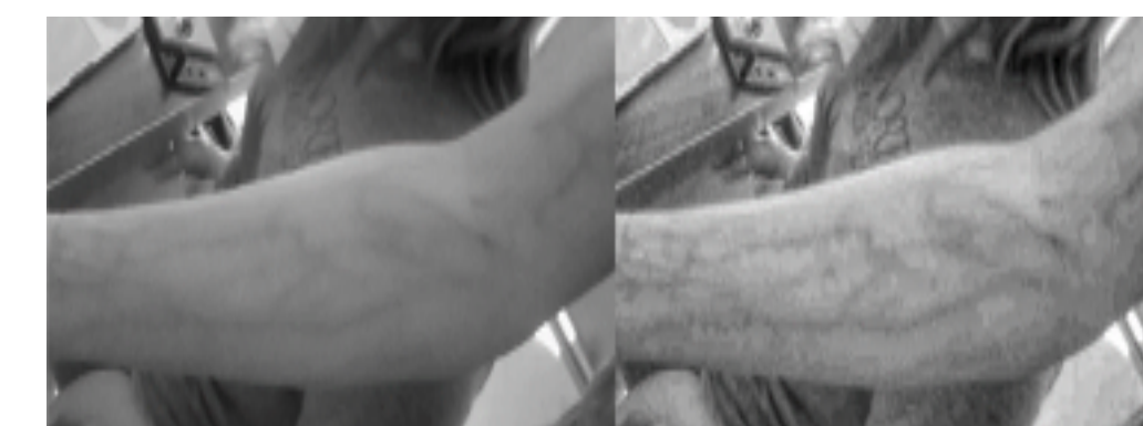
Figure 6: The image to the left demonstrates the image captured by the device. The image to the right involves the device and the use of a Laplacian filter
